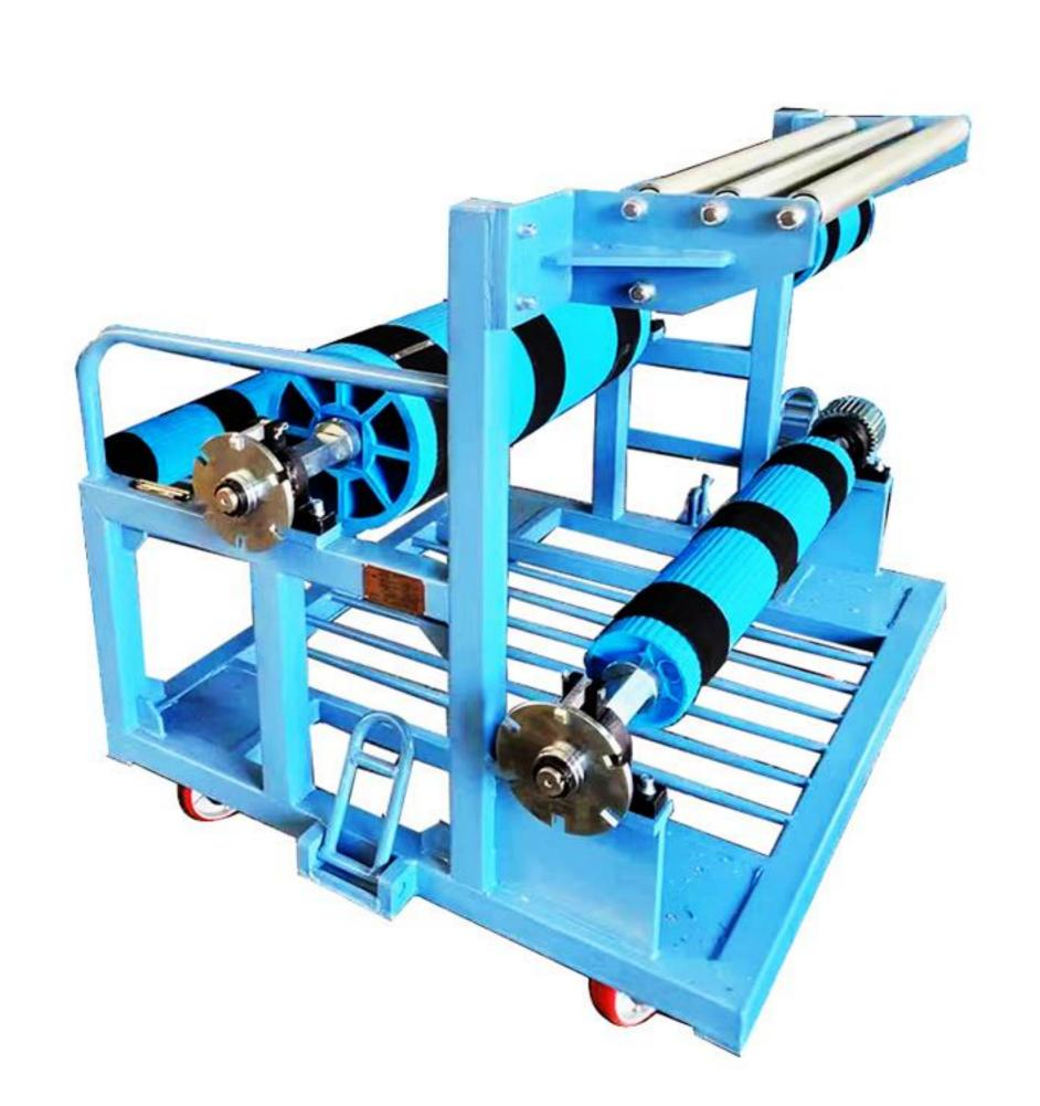
The Reel Cassette Cart is used to carry and transport tire tread, ensuring the safe and convenient transportation of tire tread during the production process.
