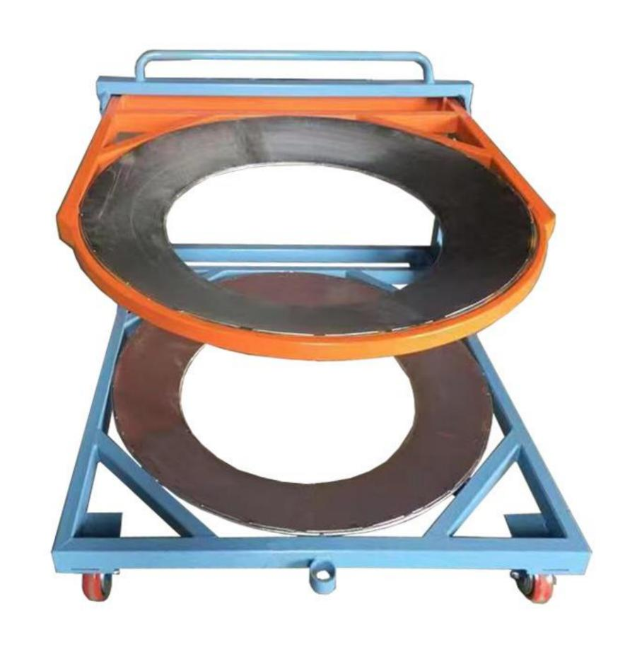
The green tire cart is a vehicle specially used to transport tire embryos, ensuring their safe and orderly flow flow and improving production efficiency.
