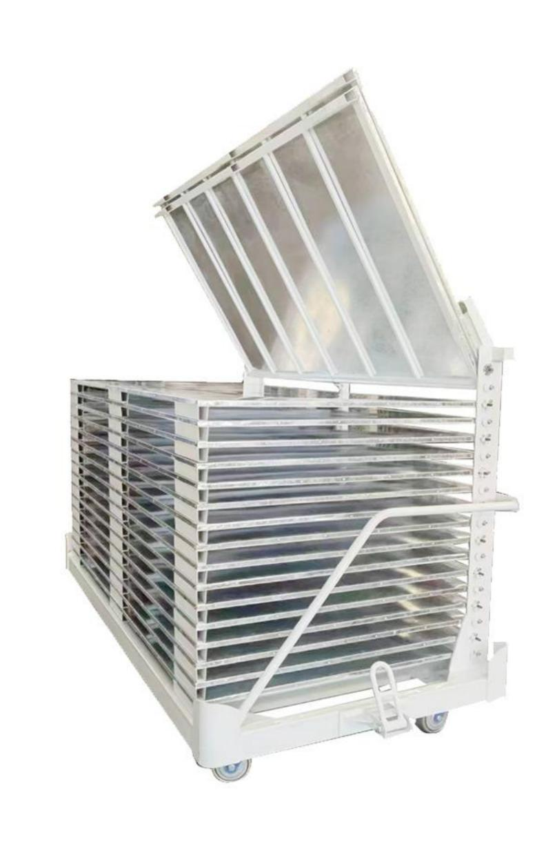
The tread tray truck features a multi-layer pallet design, making it convenient for storing and transporting rubber proucts, thereby improving the efficiency of the production process.
